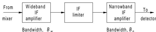
**Figure C37** Dicke-fix CFAR.
