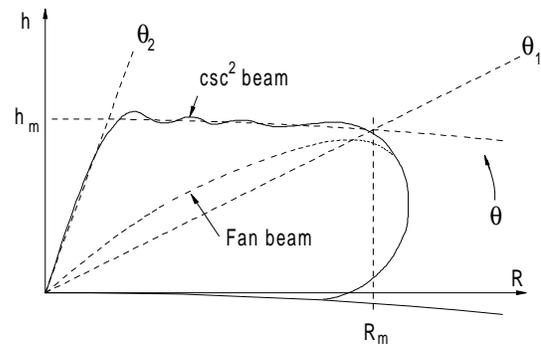
**Figure P5** Example of radar coverage using  $\text{csc}^2$  antenna (after Barton, 1988, Fig. 4.2.9, p. 163).
