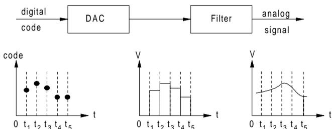
Figure C43 Digital-to-analog converter.
