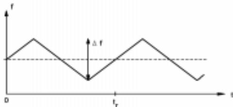
**Figure F37** Frequency deviation of sawtooth FM waveform.
