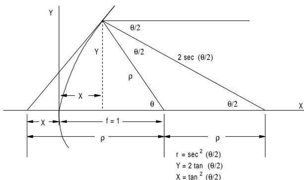
**Figure R111** Parabolic reflector (from Johnson, 1984, Fig. 17.16, p. 17.17).
