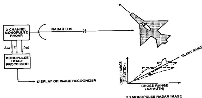
**Figure 12** Three-dimensional imaging with monopulse radar (from Wehner, 1987, Fig. 8.2, p. 343).
