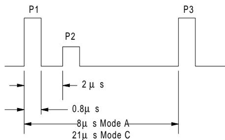
**Figure I11** Interrogation signal format (after Stevens, 1988), Fig. 3.3, p. 23.
