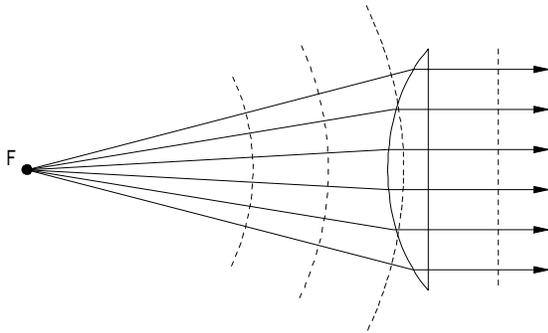
**Figure L4** Dielectric lens (after Leonov, 1986, Fig. 2.6, p. 19).
