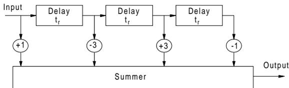
**Figure C3** Block diagram of four-pulse canceler.
