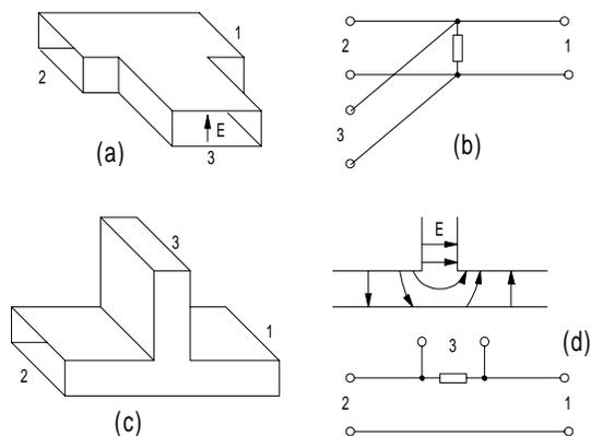
**Figure T8** Waveguide tee configurations: (a) H-plane tee, (b) equivalent circuit of H-plane tee, (c) E-plane tee, (d) equivalent circuit and fields in E-plane tee (after Lavrov, 1974, Fig. 18.43, p. 348).
