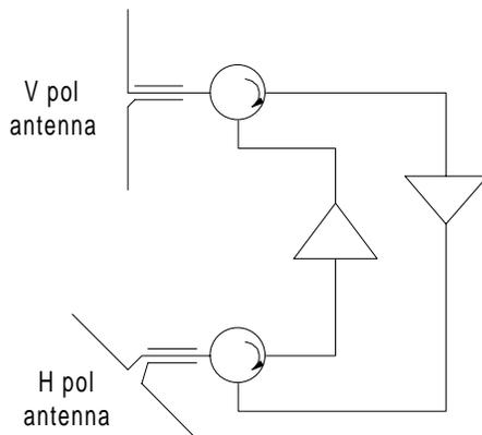
Figure E4 Block diagram of cross-pol ECM.
