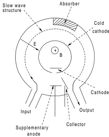
Figure A36 Annular magnetron amplifier.
