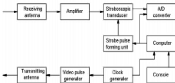
**Figure R32** Impulse radar with ultrawideband signal.
